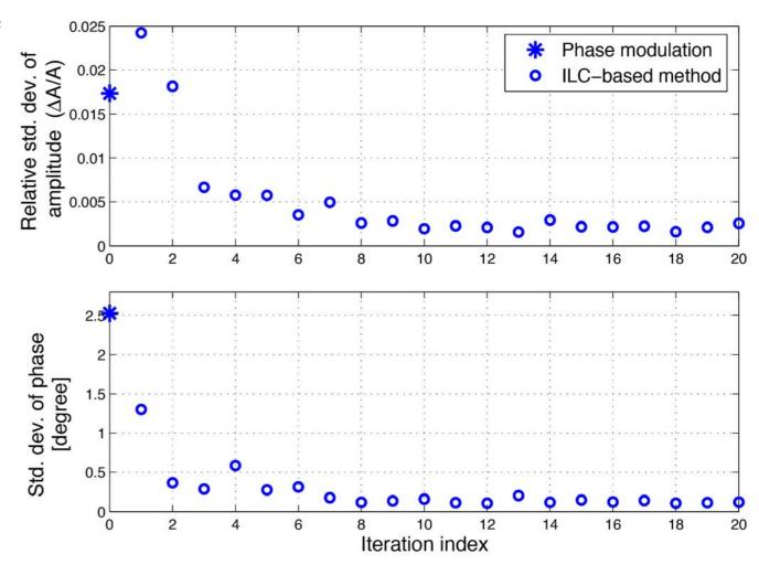
For each iteration, I and Q is measured over ten beam pulses, to suppress noise. After the input waveform is updated, the algorithm pauses for a while to let the cavity temperature re-equilibrate.
