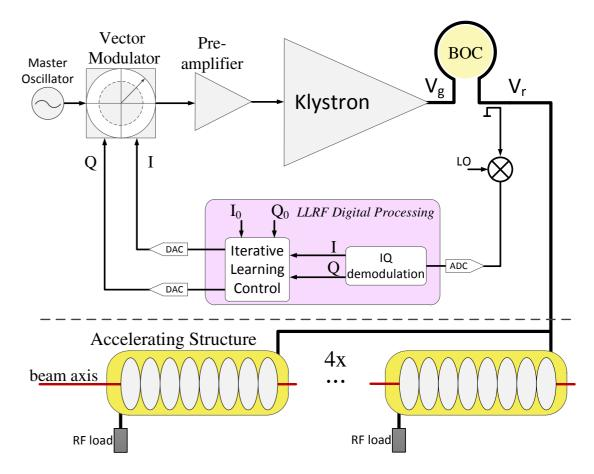
Figure 1: The simplified RF layout of a C-band RF station in the SwissFEL beamline.
